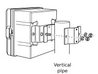
Pipe diameters: max. 62 (2.44)/min. 45 (1.77)
