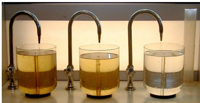
Fig. 2: Change in river-water color through the coagulation process
