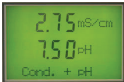
Simultaneous conductivity and pH measurement
