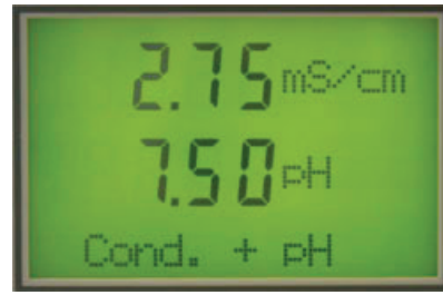
Simultaneous conductivity and pH measurement
