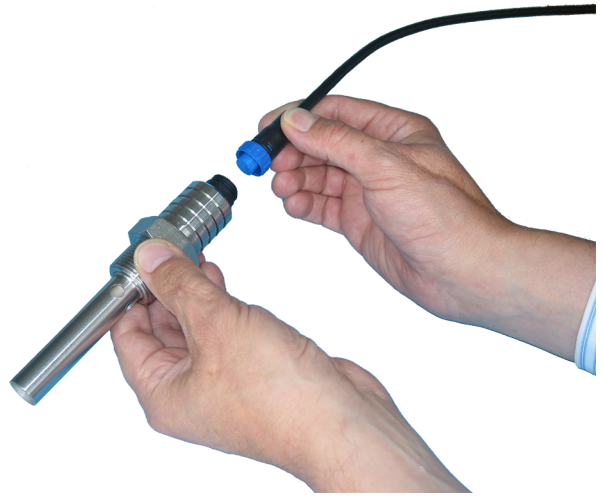
Figure 2 Detachable connector for easy installation
