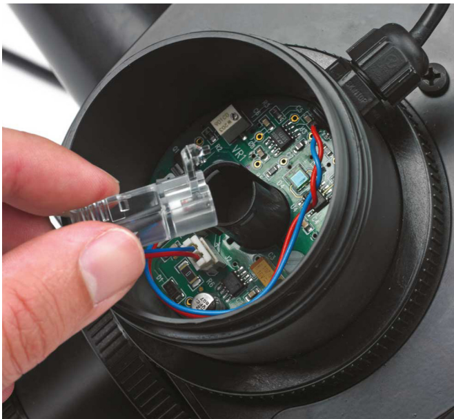
Fig. 6: Replacing the light source
